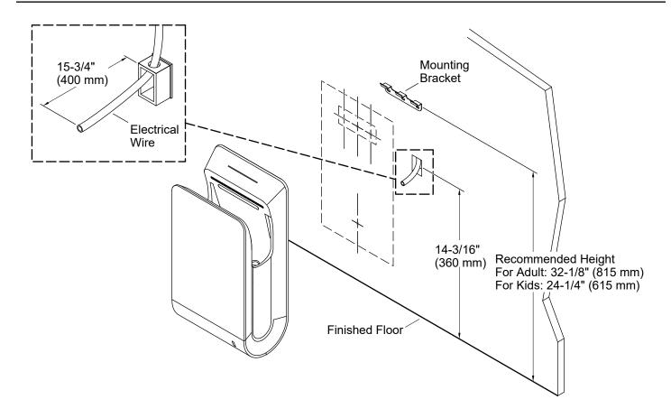
IMPORTANT! Recommend to connect the product to a single phase AC supply. Use an AWG16 wire  $(1.5 \text{ mm}^2 - 2 \text{ mm}^2)$  for connection. Keep at least 15-3/4" (400 mm) wire for connection.
