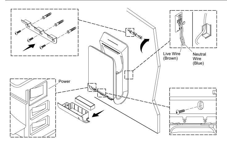
**IMPORTANT!** Verify that the hand dryer is installed at the proper location. Tighten the anti-theft screw to prevent the product from dropping onto the ground or being stolen.
